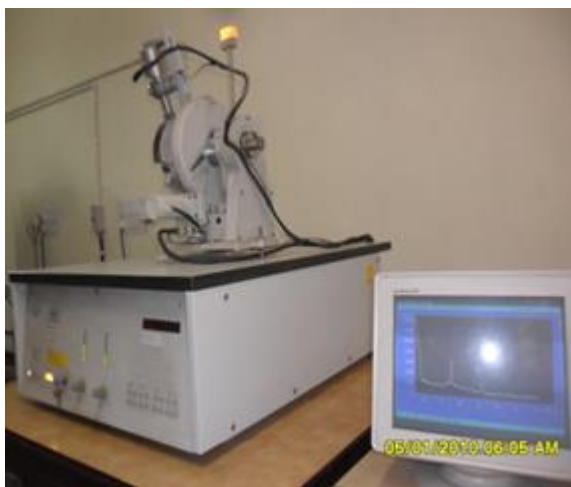
Figure 3. The X-Ray Diffraction Instrument in IEST Shibpur
