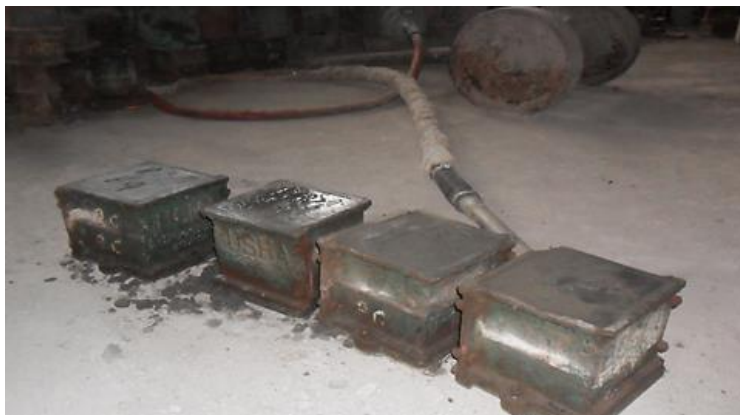
Figure 4. Cement Concrete Cube casting by compaction with Needle Vibrator
