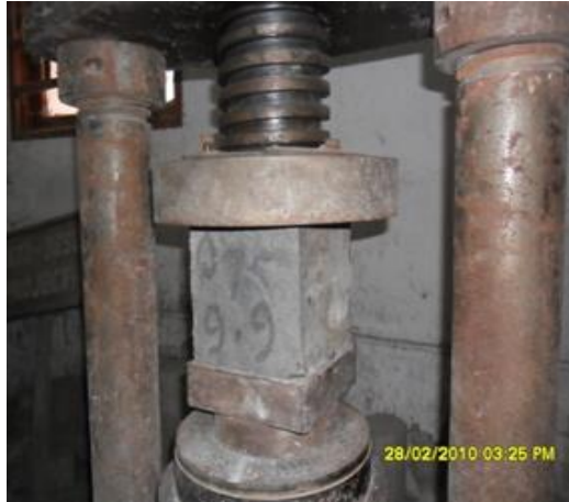
Figure 7. Compressive Strength Test being conducted.
